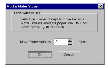
Figure 3-32. Paper Motor Test.
